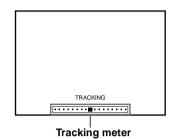
To resume automatic tracking adjustments, eject the tape and re-insert it.
